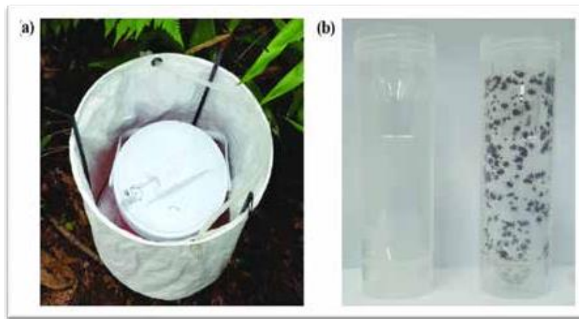
Fig 14: Dry ice bait collecting trap (a), which consists of a tarpaulin cylindrical trap and a cylindrical ice chest, installed at each environmental point and (b) a tick collection tube that prevents the escape of ticks.
